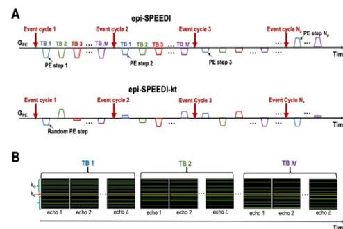
**Figure 2:** Comparison of phase-encoding schemes used in epi-SPEEDI and epi-SPEEDI-kt sequences (A) and the k-space sampling pattern in epi-SPEEDI-kt (B).  $N_{nav}$  phase lines (yellow lines) in the central k-space ( $k_c$ ) region are sampled in all the time blocks (TBs) while the outer k-space ( $k_o$ ) regions are randomly and sparsely sampled (green lines). The k-space sampling patterns are the same at the echoes in one TB but different between TBs.
