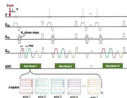
**Figure 1:** Pulse sequence design of epi-SPEEDI. The rf excitation, slice-selection gradient, phase-encoding gradient, frequency-encoding gradient, and readout are indicated by rf,  $G_{ss}$ ,  $G_{PE}$ ,  $G_{FE}$ , and ADC, respectively.  $t_{ris}$  is the time delay between the event and the first rf excitation.
