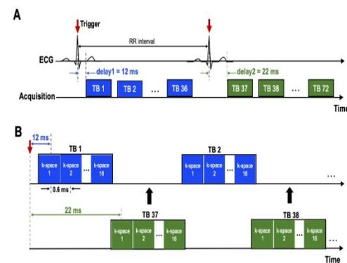
**Figure 3:** Interleaved multi-phase acquisition with two trigger delays of 12 ms and 22 ms as shown in (A) and the temporal alignment of TBs (B).
