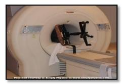
The magnetic field is not solely confined to the bore of the magnet. The stray magnetic field outside the bore of the magnet is known as the fringe field and it extends in all directions. Thus, caution needs to be taken everywhere within or around the MR scan room.
